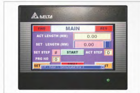
Multi-step motorized back gauge with touch screen DRO from DELTA Taiwan.
