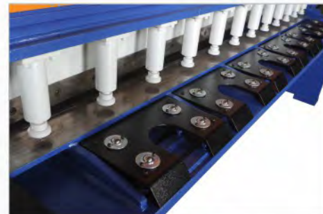
Ball Transfer table for fast and smooth handling of sheet.
